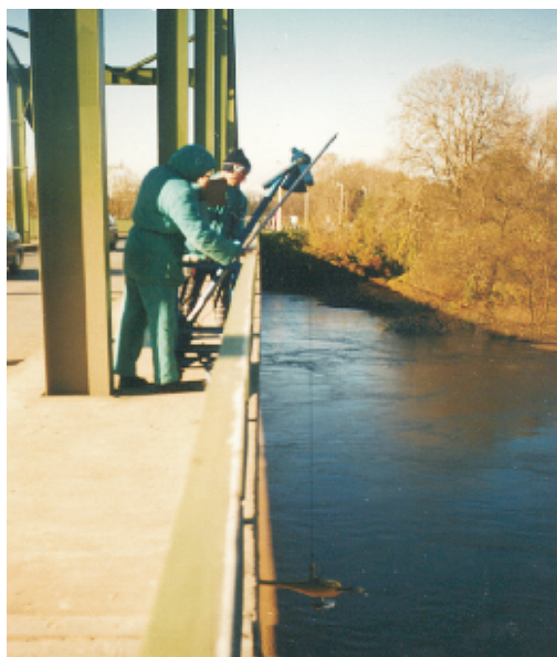
Flow measurement on the Tisza at Vasarosnameny 7th November 1998 at 9230 mm water stage
